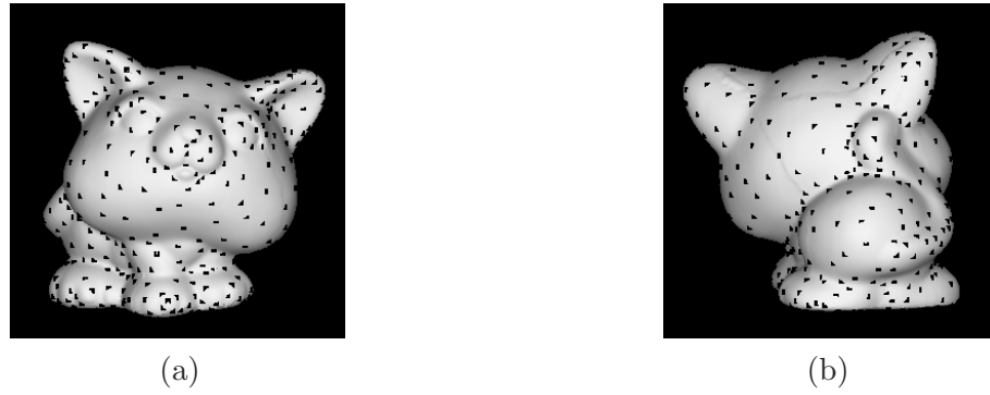
Figure 4.9 Sampling a cat model: front (a) and back (b) views of the model with a total of 550 sample vertices displayed as black dots on its surface.
